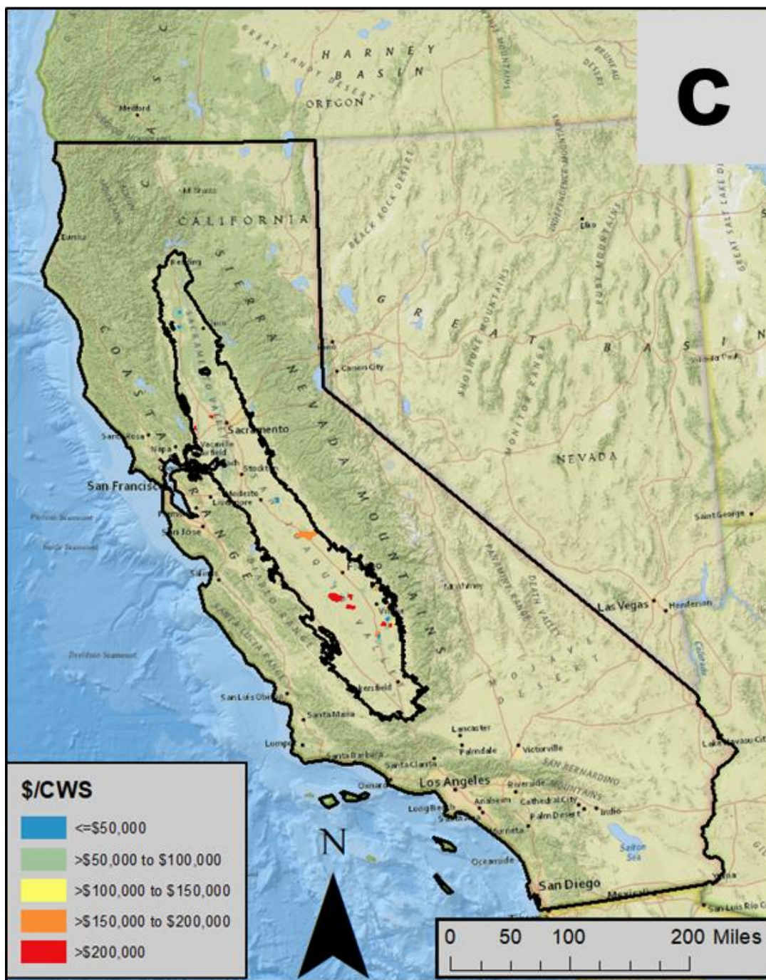
Figure 15c: Spatial distributions of impacts and costs for CWS wells with a 1.0 drought factor: costs for additional pumping lift. Tallies by buffered CWS service area.
