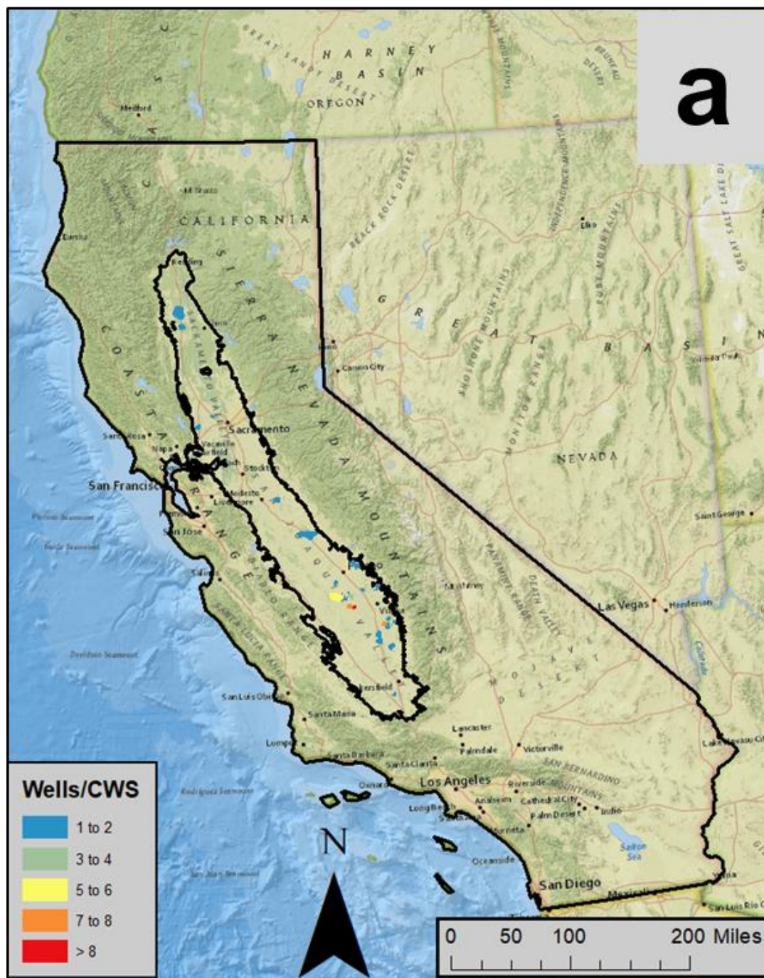
Figure 15a: Spatial distributions of impacts and costs for CWS wells with a 1.0 drought factor: impacts other than additional pumping lift (pump lowering, well screen rehabilitation, well replacement). Tallies by buffered CWS service area.
