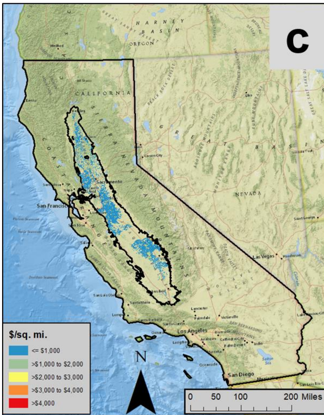
Figure 10c: Spatial distributions of impacts and costs for domestic wells with a 0.5 drought factor: costs for additional pumping lift. Tallies by PLSS section.
