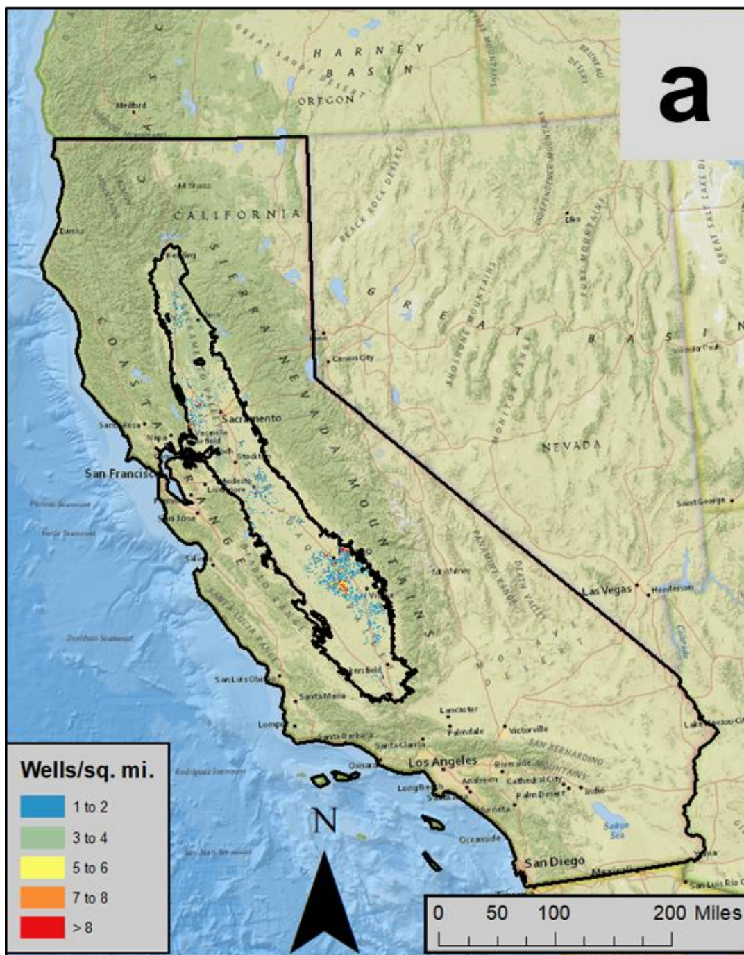
Figure 12a: Spatial distributions of impacts and costs for domestic wells with a 1.0 drought factor: impacts other than additional pumping lift (pump lowering, well screen rehabilitation, well replacement). Tallies by PLSS section.
