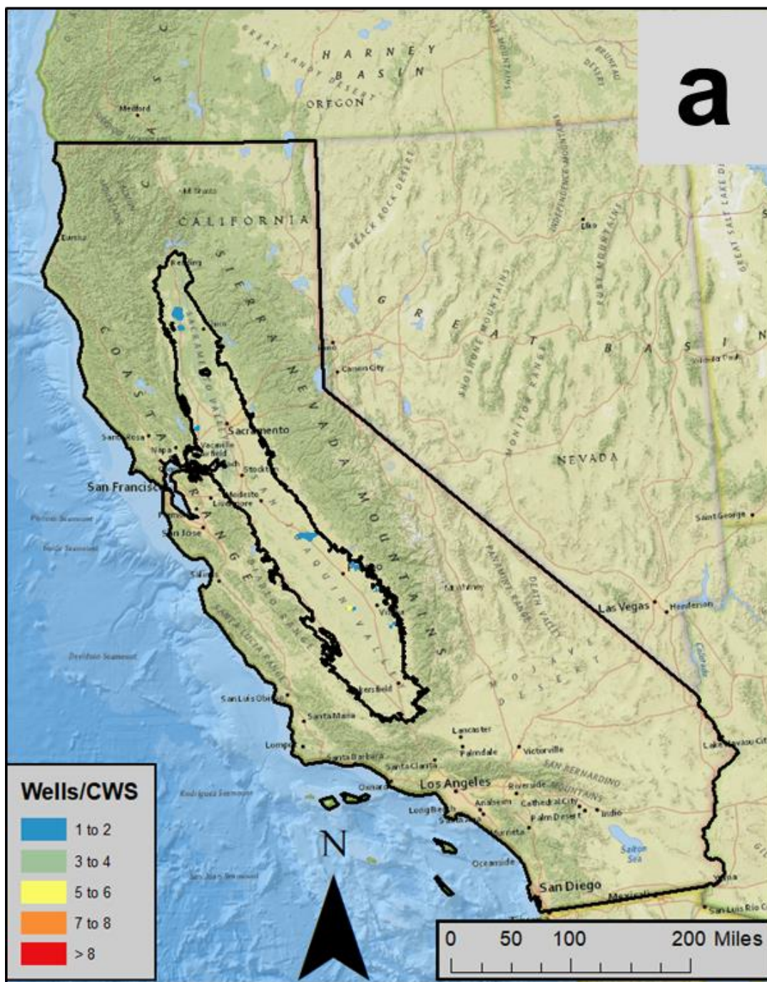
Figure 13a: Spatial distributions of impacts and costs for CWS wells with a 0.5 drought factor: impacts other than additional pumping lift (pump lowering, well screen rehabilitation, well replacement). Tallies by buffered CWS service area.
