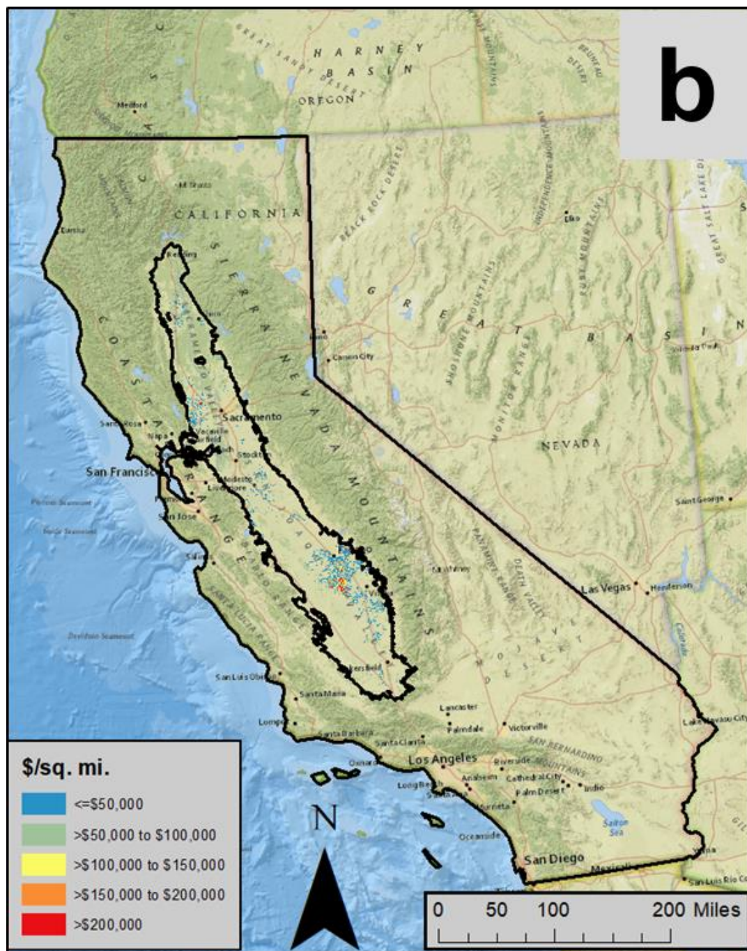
Figure 11b: Spatial distributions of impacts and costs for domestic wells with a 0.75 drought factor: costs for impacts other than additional pumping lift. Tallies by PLSS section.
