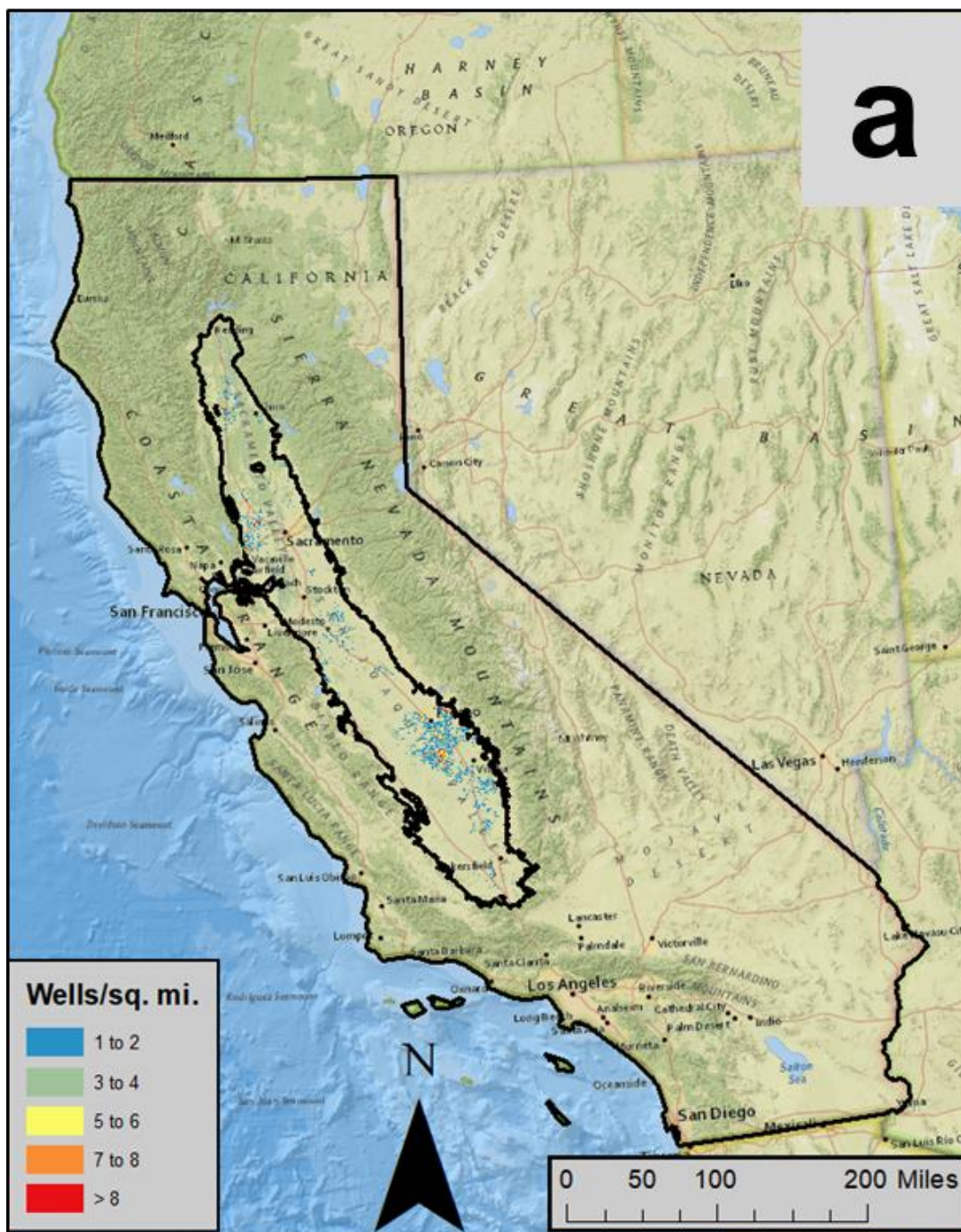
Figure 11a: Spatial distributions of impacts and costs for domestic wells with a 0.75 drought factor: impacts other than additional pumping lift (pump lowering, well screen rehabilitation, well replacement). Tallies by PLSS section.
