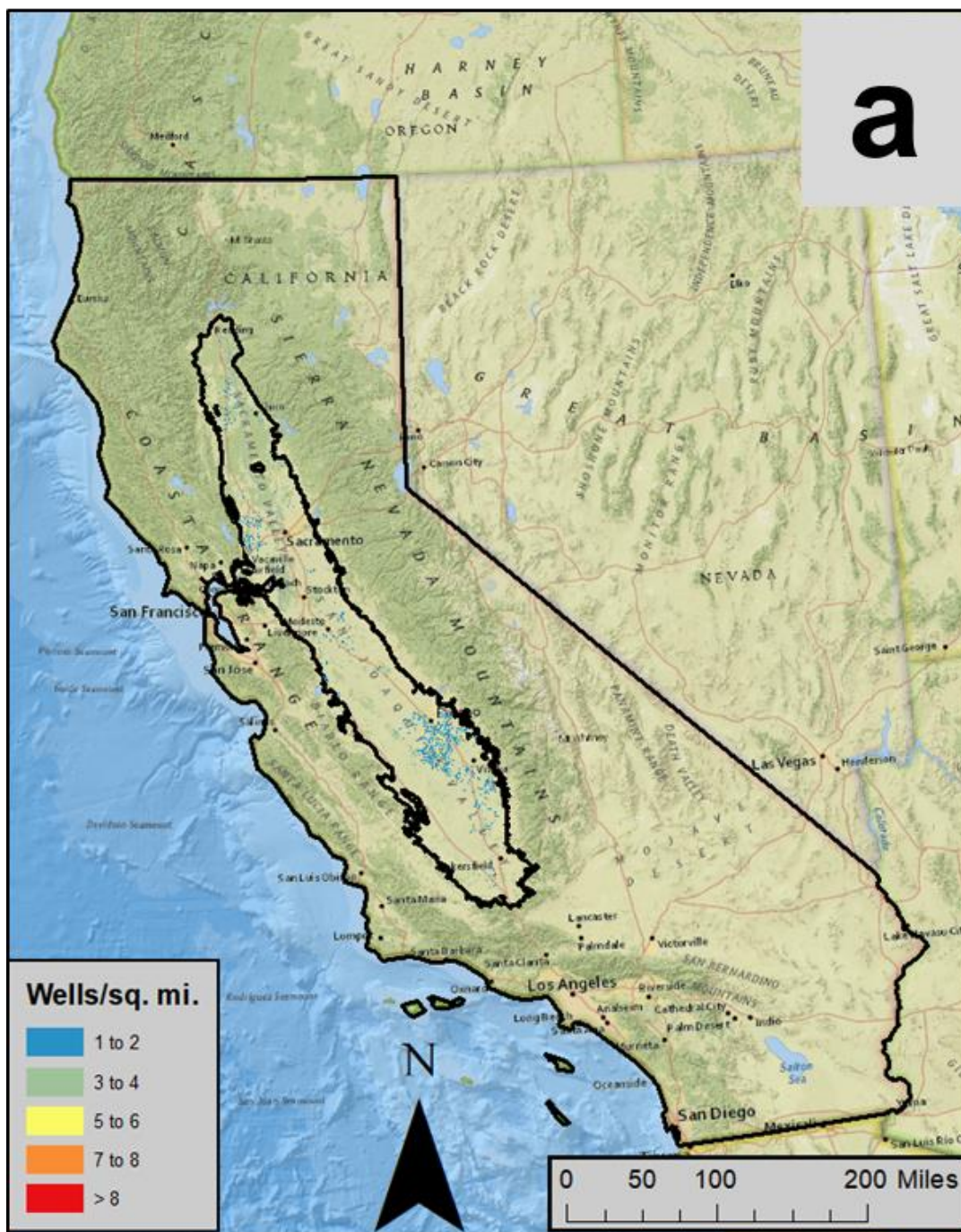
Figure 10a: Spatial distributions of impacts and costs for domestic wells with a 0.5 drought factor: impacts other than additional pumping lift (pump lowering, well screen rehabilitation, well replacement). Tallies by PLSS section.
