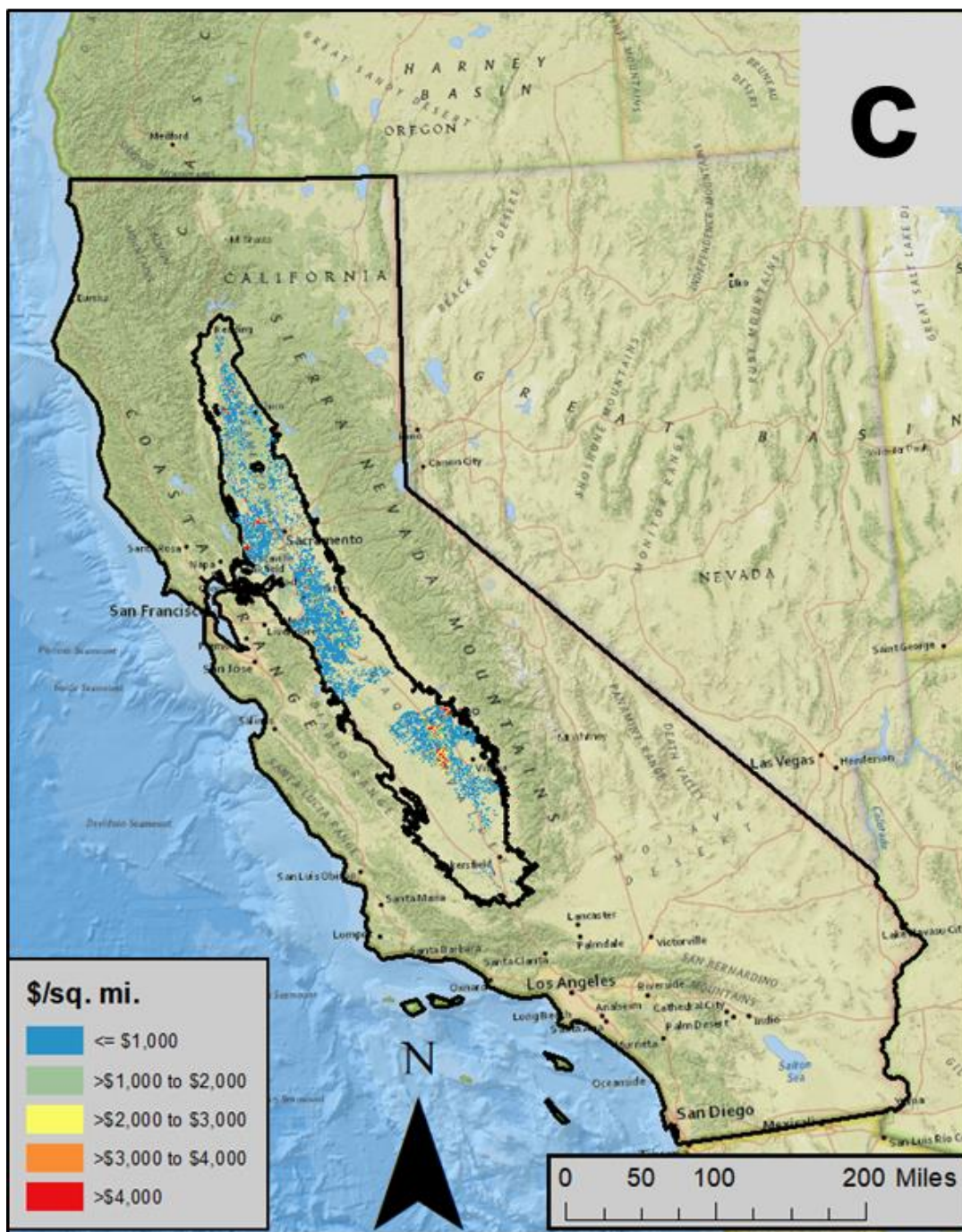
Figure 12c: Spatial distributions of impacts and costs for domestic wells with a 1.0 drought factor: costs for additional pumping lift. Tallies by PLSS section.
