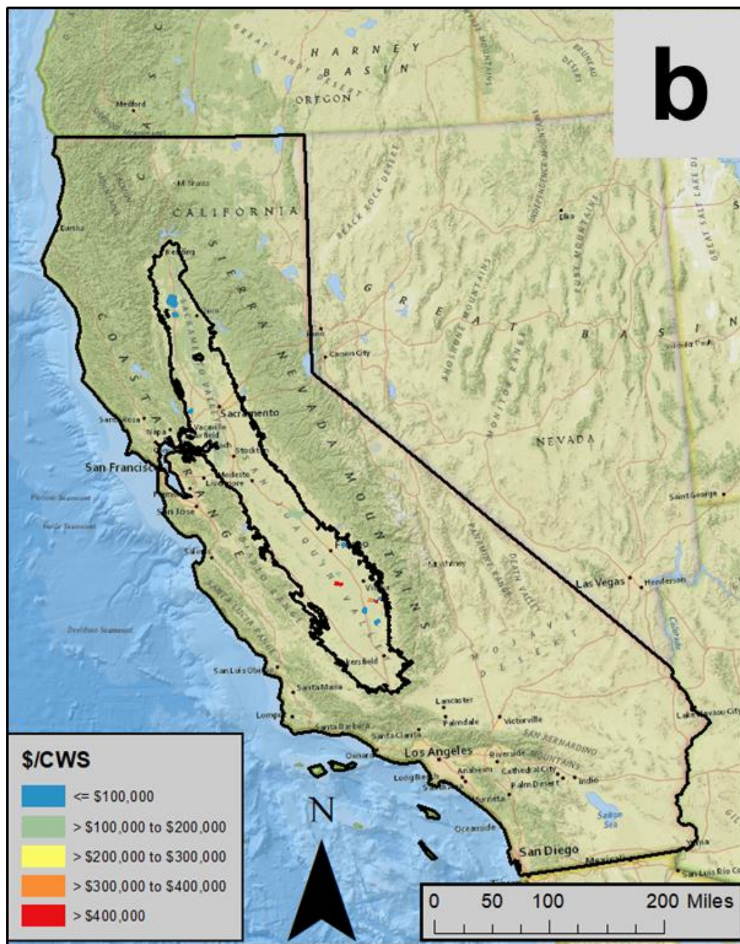
Figure 14b: Spatial distributions of impacts and costs for CWS wells with a 0.75 drought factor: costs for impacts other than additional pumping lift. Tallies by buffered CWS service area.
