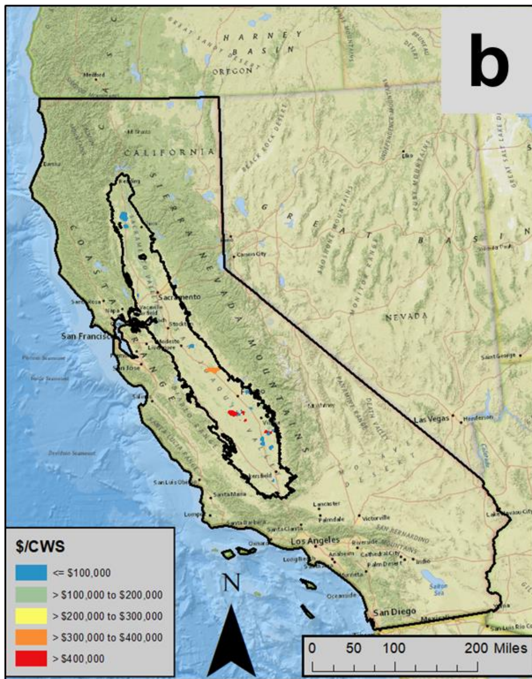
Figure 15b: Spatial distributions of impacts and costs for CWS wells with a 1.0 drought factor: costs for impacts other than additional pumping lift. Tallies by buffered CWS service area.
