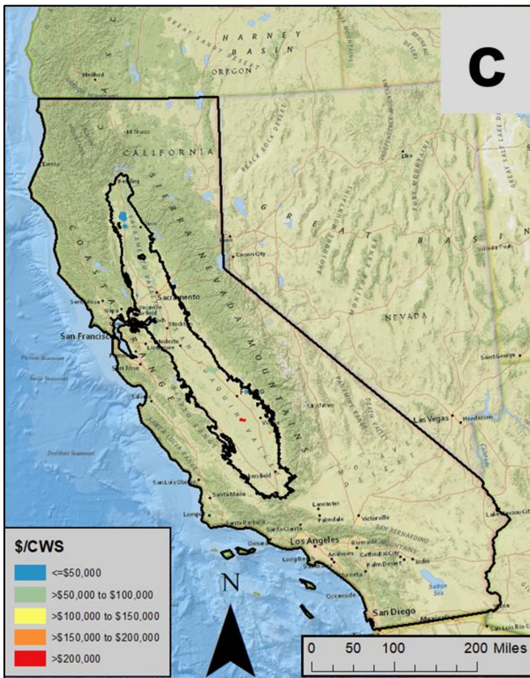
Figure 13c: Spatial distributions of impacts and costs for CWS wells with a 0.5 drought factor: costs for additional pumping lift. Tallies by buffered CWS service area.
