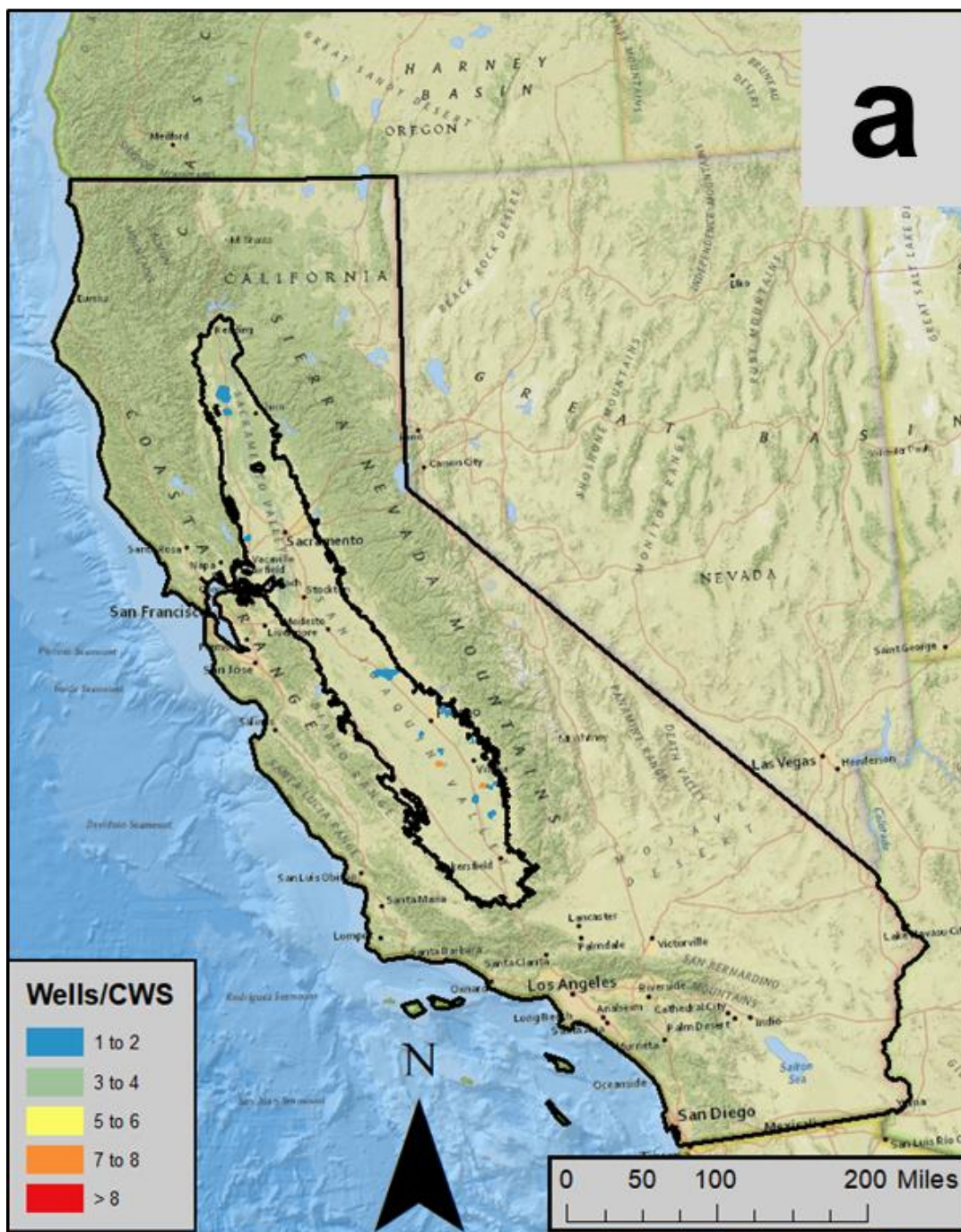
Figure 14a: Spatial distributions of impacts and costs for CWS wells with a 0.75 drought factor: impacts other than additional pumping lift (pump lowering, well screen rehabilitation, well replacement). Tallies by buffered CWS service area.
